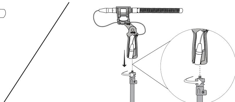
**Rycote® Softie Lyre Mount with Camera Clamp Adapter for VP89M and VP89S**
